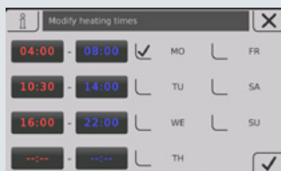
Fig. 2 View of the heating times (individually adjustable)
